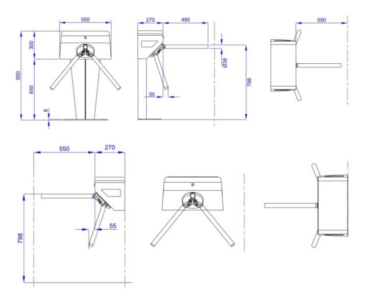
Concrete Base to specification at least fck (cube)  $300N/mm^2$  of resistance. Base to be flat and level to +/- 5mm over footprint area. Dimensions to be > 700 x 500 x 150 deep min for pedestal-mounted version (units in mm).
