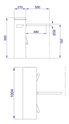
Important: Any horizontal pipe or conduit running below the Tripod Turnstile must be at least 140mm below FFL. Metal conduit for cables should be raised at least 50mm from foundation. It is the customer's responsibility to ensure the structural integrity and strength of the installation location. The dimensions given in this Product Data Sheet are for information only. In order to prepare the installation site, please refer to your usual Gunnebo Customer Service contact.
